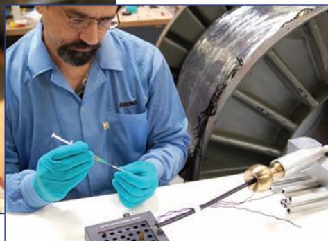
*(Left) Strength member's armored wires meticulously bent around the mechanical insert to optimize mechanical load-bearing capabilities.*
